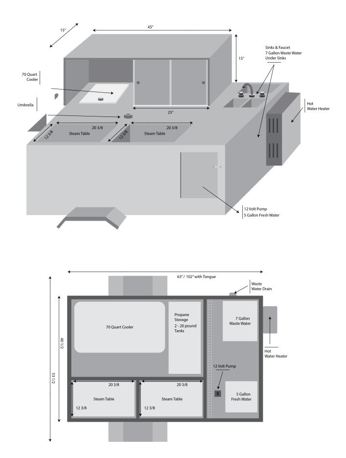
Our NEWEST hot dog cart, The Cater Pro boasts a two commercial steam tables with dual cast iron burners and controls for each. Boil and steam all on the same cart.
